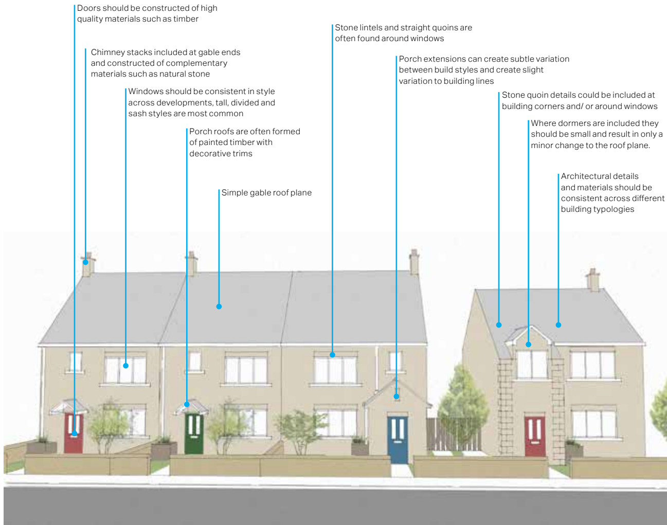
Figure 91: Illustration of ways which modern development can incorporate materials and architectural details that fit the local vernacular
